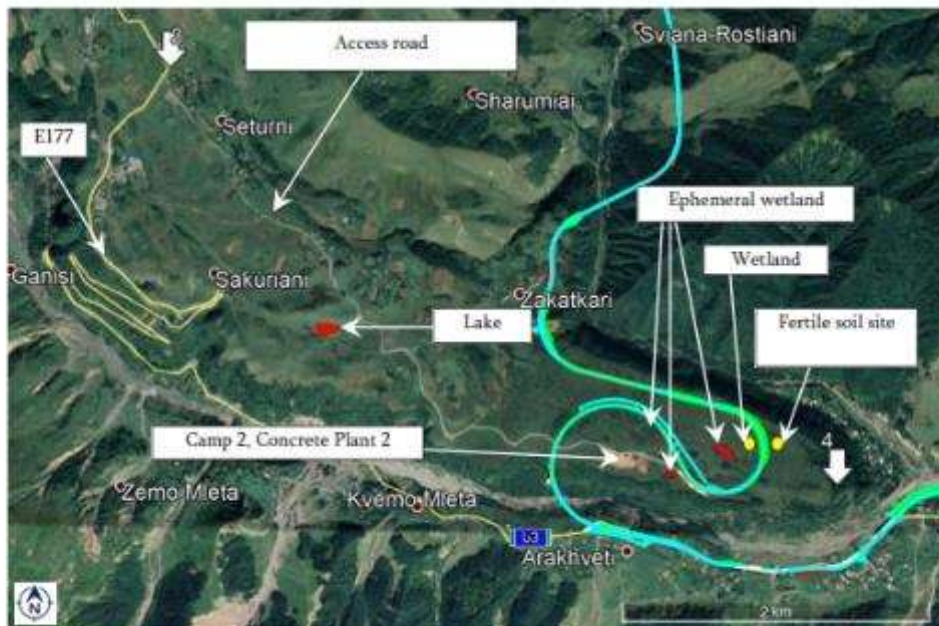
Figure 18. Section II along with the existing highway (E117), Access road, project infrastructure and sensitive sites (arrows indicate the starting and the last points of the section)
