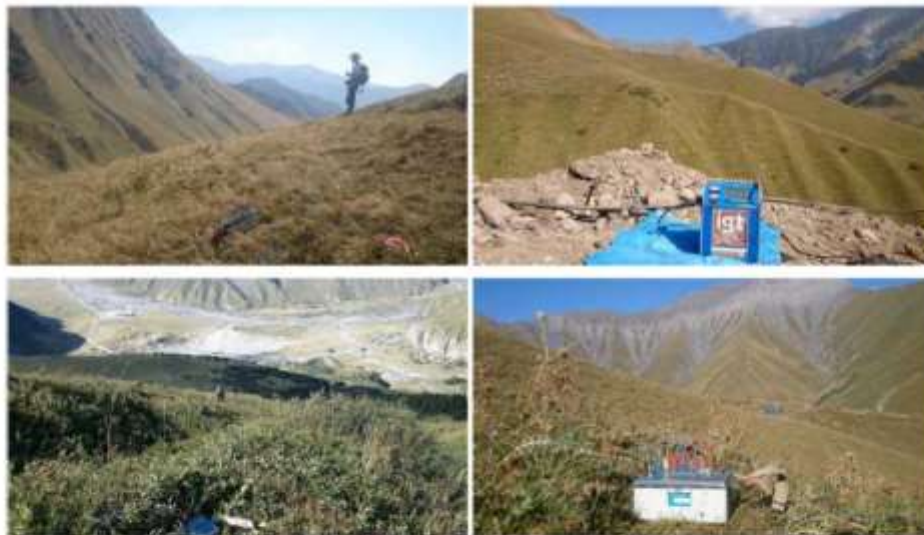
Figure 3 Deep ERT surveys along Gudauri Tunnel
